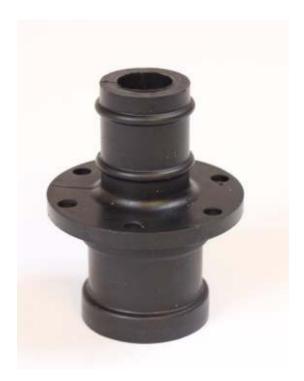
Kea-Flex makes this split pipe seal which is supplied to James Walker UK Ltd. It manufactures the single cavity tool in house and the part is produced on a compression press in black Neoprene 40 Shore A.
